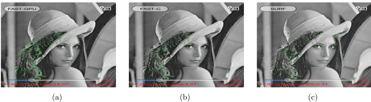
Fig. 5: The results of corner detection after using (a) FAST-GPU; (b) FAST-CPU; (c) SURF-CPU
